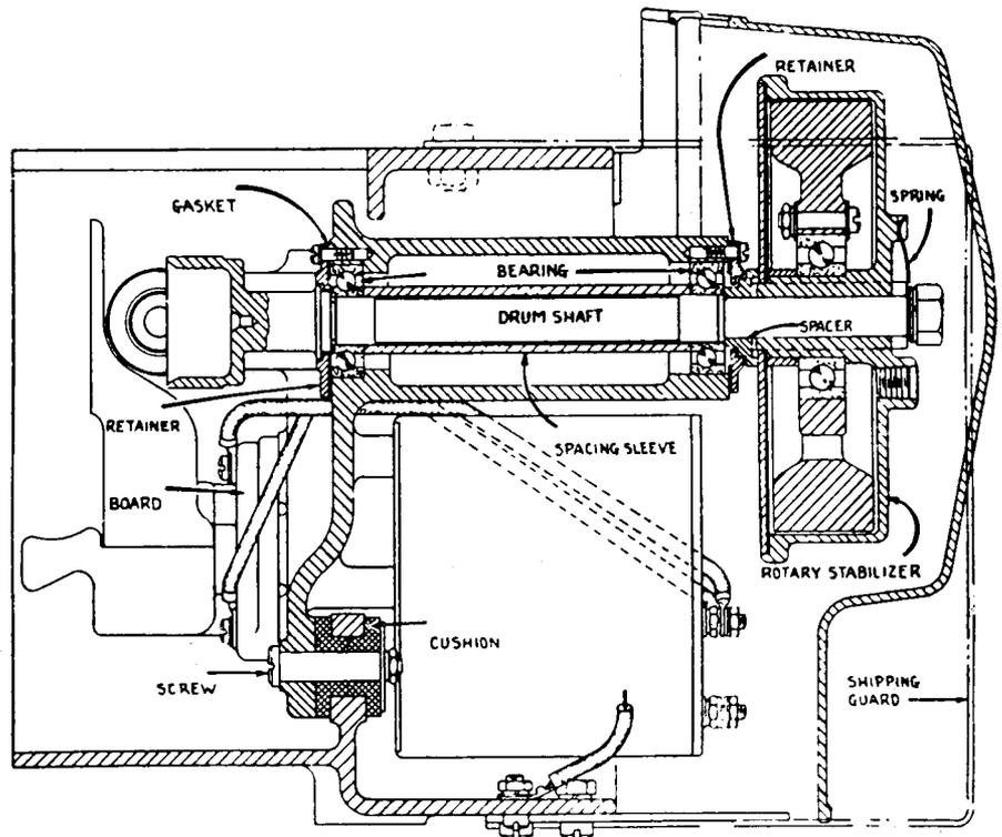
Rotary stabilizer construction of F. J. Loomis and E. W. Reynolds.
