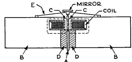
Fig. 11. Cross section of improved recording galvanometer, G. L. Dimmick. A—armature; B,B—pole pieces; C,C—working air gaps; D,D—nonmagnetic spacers; E—tensioned bronze ribbon.
