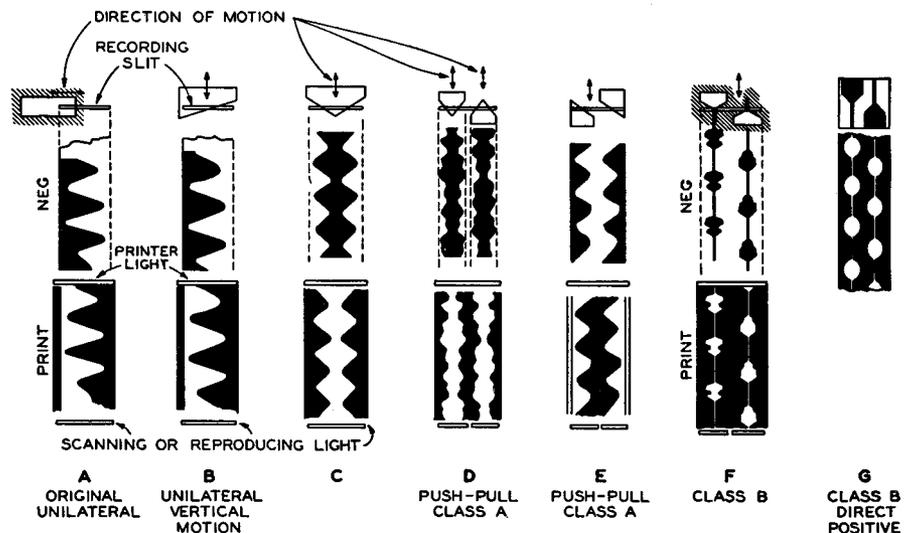
Fig. 14. Variation types of area soundtracks, and light-spot shapes which produce them.
